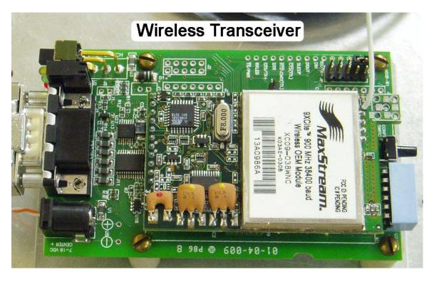
The wireless transceiver is another integral part of the wireless drifter. This is the component which allows the drifter to transmit data to a pc so that it can be interpreted. The particular chip used is the Maxstream 9XCite (www.maxstream.net) which supports the following features, as well as many others:
