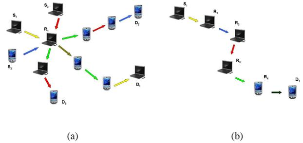
Fig. 5. a) Switching delay at relay node  $R_1$  due to multiple communication flows ( $S_1 \rightarrow D_1, S_2 \rightarrow D_2, S_3 \rightarrow D_3$ ):  $R_1$  becoming bottleneck; b) Switching delay along one single communication flow due to multiple relay nodes operating over different frequency channels
