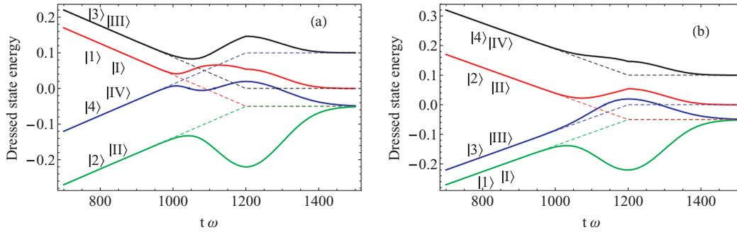
FIG. 9. (Color online) Nondegenerate model: Dressed state energies (solid lines) and bare state energies (dashed lines) as a function of time for the positive (a) and negative (b) Stokes chirp;  $\Omega_3(t_0) = 0.7$  (respective effective pulse area  $A \simeq 5.9\pi$ );  $|\alpha'|/\tau_0^2 = 10$ .
