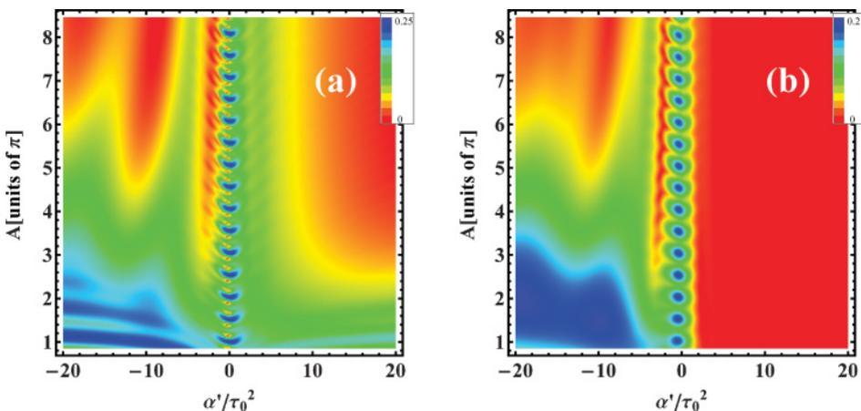
FIG. 6. (Color online) Nondegenerate model: Density plot of averaged coherence for the resonant (a) and off-resonant (b) systems as a function of the effective pulse area,  $A$ , and chirp parameter,  $\alpha'/\tau_0^2$ .
