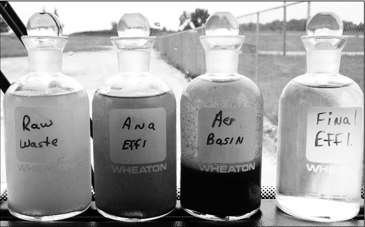
The steps of the wastewater treatment: from start to finish.
