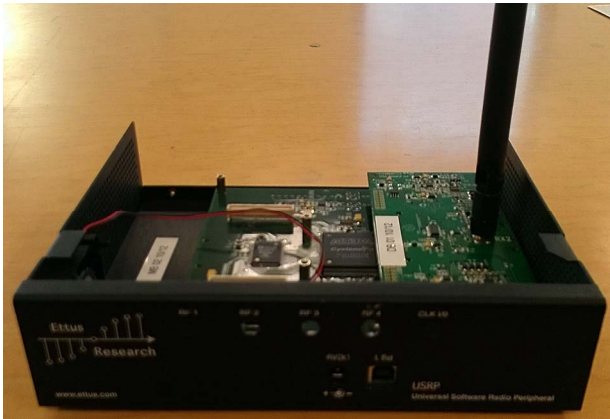
Fig. 6. Ettus Research USRP1 with RFX 900 TX/RX.
